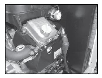
Figure 28. Checking Ignition Spark
